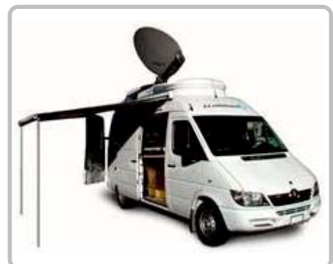
Sliding tents are provided at lift as shown and rear side of the vehicle for convenience of operation staffs. Rain as well as strong sun ray protections.
