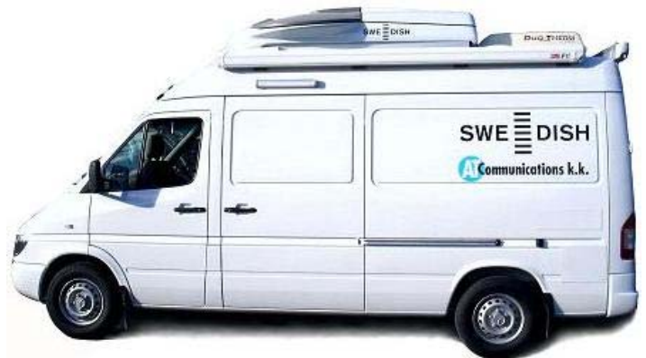
Side view. Air-conditioning unit is seen on the rooftop beside SWE-DISH DA-150 Ku-band antenna system.
