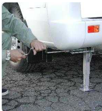
Two stabilizers at rear left and right kill springs of the vehicle so that transmission could be made stable. An indicator is provided at driver's panel alarming when stabilizers are in
